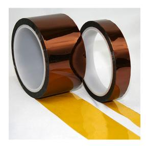
This tape consists of a polyimide film and silicone adhesive designed for high temperature masking applications, including protecting printed circuit board gold finger contacts during wave soldering. It is used in electrical insulation applications meeting class H requirements. Thin and conformable enabling masking of uneven surfaces.
